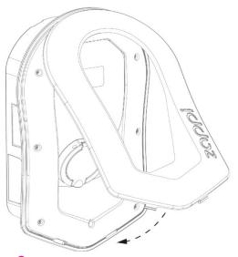
**Step 2:** Add fascia to the enclosure cover of the zappi as shown.
