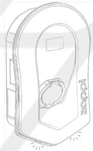
Step 3: Ensure the 2 tabs at the bottom of the fascia click to indicate its securely fixed in place.
