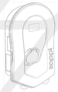
**Step 3:** Ensure the 2 tabs at the bottom of the fascia click to indicate its securely fixed in place.
