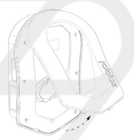
**Step 1:** Carefully remove fascia from the zappi by pressing the 2 clips located at the bottom of unit inwards whilst pulling the fascia towards you.
