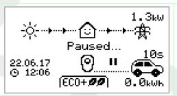
zappi is paused for a few seconds in order to limit the start/stop frequency during ECO+ mode charging.
