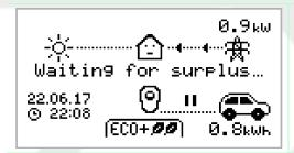
zappi is waiting for sufficient surplus power from the microgeneration system. This screen will be shown in ECO+ mode as it is only in this mode that charging will stop if there is not enough surplus power.
