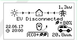
The EV is not connected to zappi.
